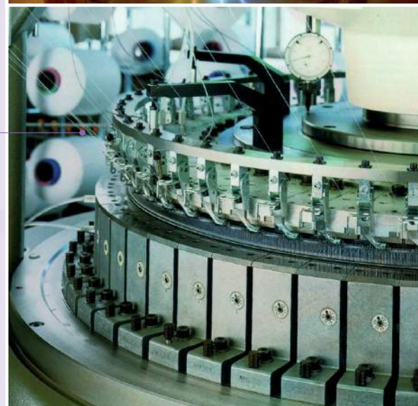
Example of application: Functional check of a circular knitting machine during running operation.
